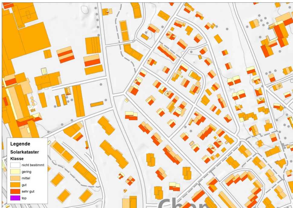
Figure 7.1.5: Solar cadastre which is available as source for calculating the solar photovoltaics and heat potential.
